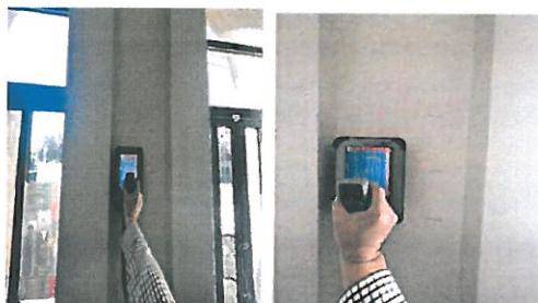
1) RADAR STALPI S1 - PARTER - BETON ARMAT
