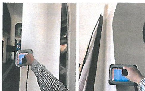
2) RADAR STALPI PARTER S2 - ZIDARIE
